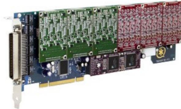
The TDM2400P is a mother board with space for a total of six analog modules. Each of the modules provides four analogue channels (4xFXO or 4xFXS). The following combinations are available:
