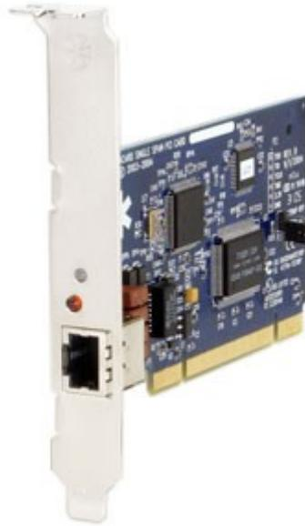
The TE110P (E100P, T100P) is a 1-Port T1/E1 card. The card has a jumper that lets you choose whether the card should work in the T1 or the E1 mode. Please set the jumper accordingly. This jumper is not present on the older, obsolete E100P and T100P cards because a different card exists for each mode. Install the card in an empty PCI slot and restart your system.
