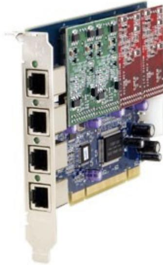
The TDM400P is a mother board with space for a total of four analog modules. Each of the modules provides one analogue channel. The following combinations are available:
