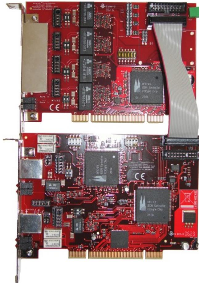
The order of the PCI cards is very important regarding the Master/Slave settings. The order is defined by how you have entered the PCI card into the Computer and how the mainboard has wired the PCI Slots. In general it is not known how the order will be.
