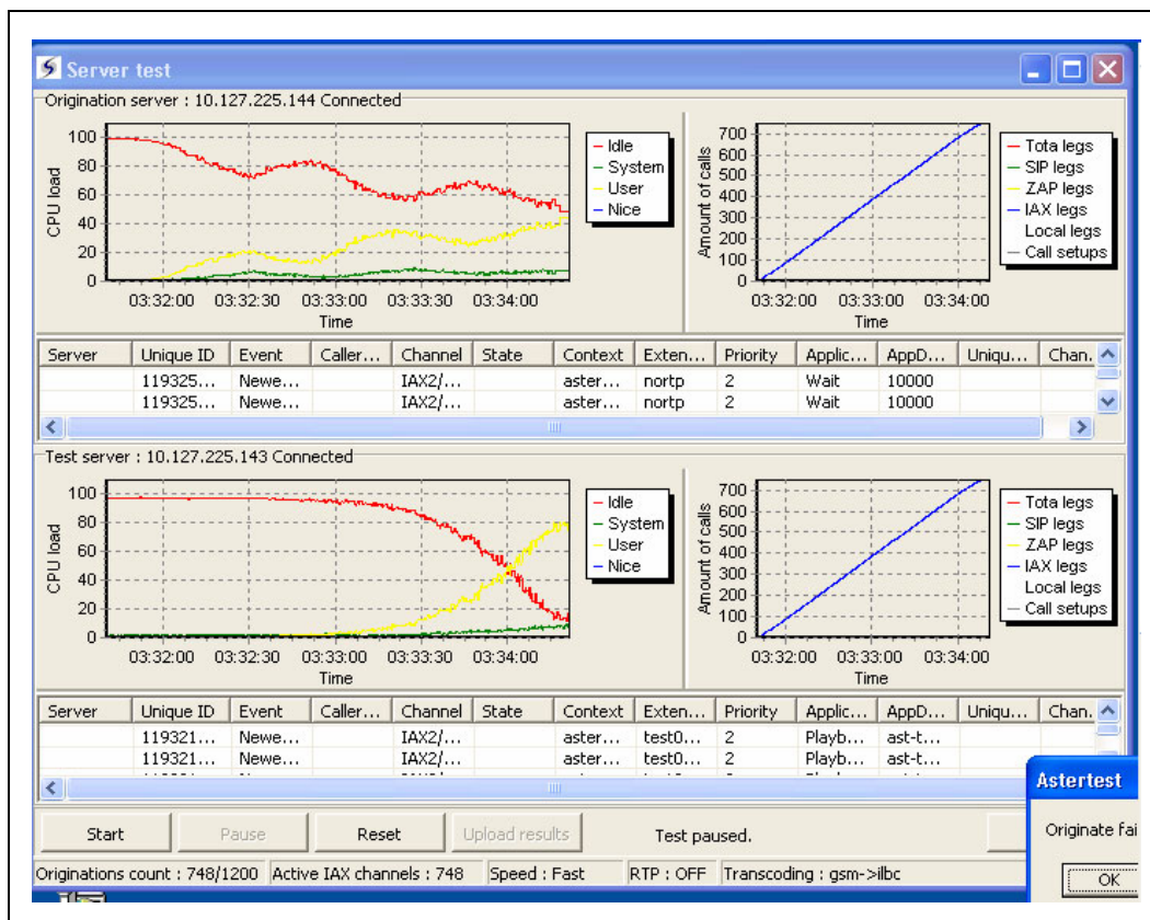
Figure 3. Astertest on Dual Quad-core at 2 GHz, GSM->iLBC Transcoding (ICC Compiler)
